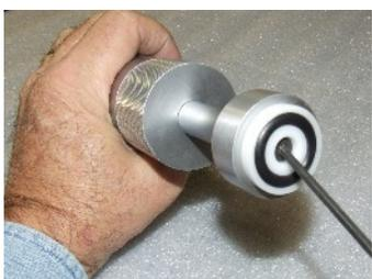
11. Install the piston pad holder then the springs and piston pad. The springs will locate in the small recesses machined into the pad and pad retainer. Use a small amount of grease to help hold the springs in place during assembly.
