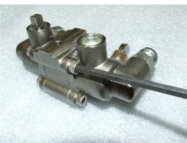
9. Attach the valve body to the spacer block. Take care not to distort the o ring seal. Snug, but do not tighten, the bolts until after the coupler shaft is installed.
