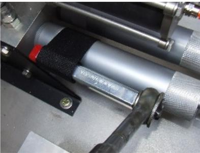
2. Loosen and remove the metering cylinder by rotating it counterclockwise. Do not use a pipe wrench! Use a strap wrench.
