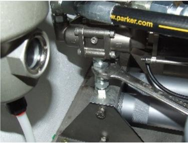
3. Use a 7/8" wrench to loosen the fittings at the COCO spacer block. Do the same for the "A" and "B" sides.
