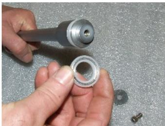
9. Be sure to install the seals with the metal springs facing out, towards the piston seal retainer.
