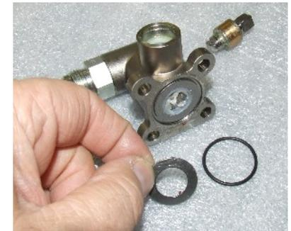
**Cleaning** Clean the components thoroughly, but do not use steel bristle brushes or instruments likely to scratch or gouge. Most solvents and cleaning agents can be used without damage to the stainless steel parts.
