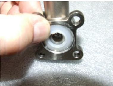
6. Install the exterior seal (S-332) with the spring groove facing away from the ball.
