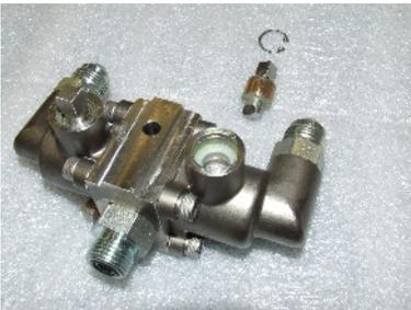
7. Remove the coupler shaft along with it's bushing and set aside.
