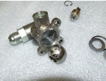
12. Now the ball can be removed from the housing. Inspect the ball looking for wear or scratches in the surface. Replace if needed.
