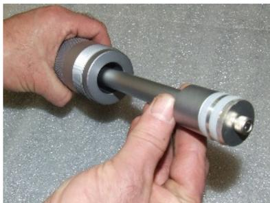
5. Now the piston can be removed from the metering cylinder.
