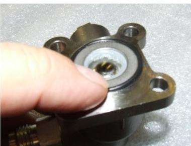
8. Press a new o-ring into the groove around the outside of the spring and washer. Use silicone lube to hold it in place.
