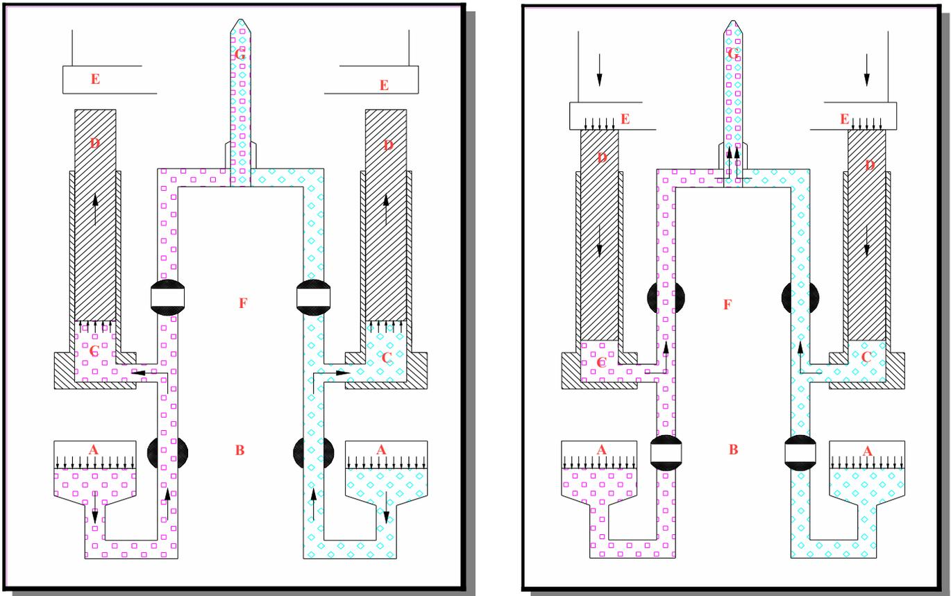
The resin components are pressurized within vessels (A) or by pumps. Pressurized, the components flow through open inlet valves (B) to enter their respective metering cylinders (C).
