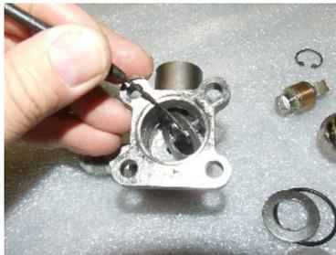
14. Using the seal pick remove the flat washer
