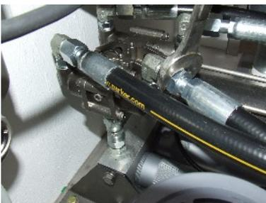
1. Using a 7/8" wrench, remove the inlet and outlet hose from their respective fittings at the COCO valve.
