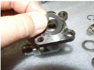
1. Fit the seal spring (S-330) into the pocket with its concave side toward the ball. 12. Remove the lower
