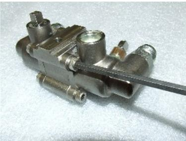
5. With a 3/16" Allen wrench, remove the four bolts that hold the ball valve body to the spacer block.
