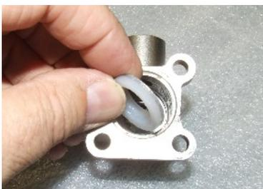
3. Insert the seal perpendicular to the bore until it is within the pocket. Then, twist it flat so that the spring side of the seal is facing down.
