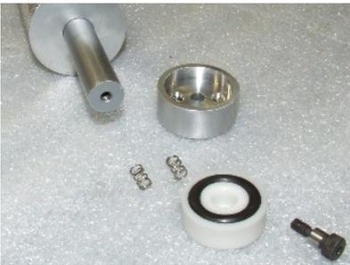
3. Remove the piston pad, springs, and piston pad holder from the metering piston. Be careful not to loose the springs.
