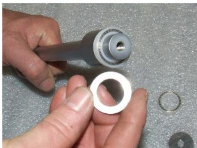
7. Seal spacer removed.
