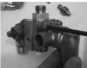
9. Attach the valve bodies to the Coco Spacer Block (M-572). Take care not to distort the o ring seals. Snug, but do not tighten the bolts!
