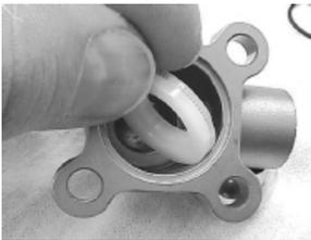
3. Insert the seal vertical to the pocket until it is within the pocket. Then, twist it flat so that the spring side of the seal is facing down.
