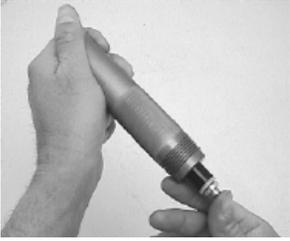
7. Lubricate the piston and chamber with silicone and insert the piston pad end first into the bottom (threaded end) of the metering cylinder.
