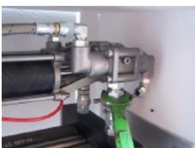
3. Use a 7/8" wrench to loosen the JIC fittings at the base manifold unions. The COCO ball valve assembly can now be removed from the cabinet for further disassembly.
