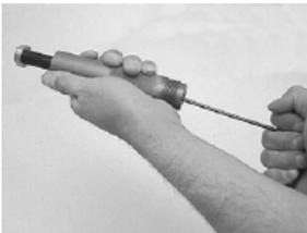
1. Press the metering piston from the cylinder bore. If it is seized, phone Lily or visit a machine shop for assistance. Do not damage the bore!
