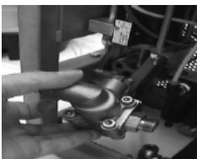
15. Fit the valve assembly to its frame. Make certain that the valve spline fits snugly into the frame slot. Apply an anti-seize compound to the threads of the mounting bolt (S-334) and draw it up tight.
