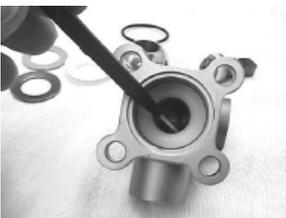
11. Use the seal pick to gently urge the lower seal from its seat. Take care not to scratch the housing.
