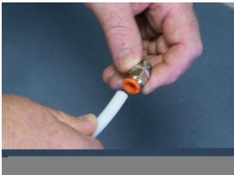
The Pneumatic fittings used throughout the dispenser are of the “press-to-connect” variety. The connection is made by firmly inserting or pressing the tube into the fitting. The tube is released by holding the fitting collar firmly back against the fitting body, while pulling the tube from the fitting.
