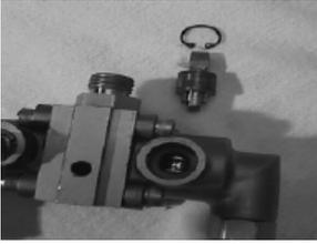
5. To remove the snap ring, grasp the coupler shaft (M-581) with a cushioned tool, and gently work it and its bushing (M-802) from the cavity.
