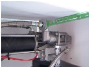
1. Use an 11/16" wrench to remove the inlet and outlet hose fittings at the COCO valves.
