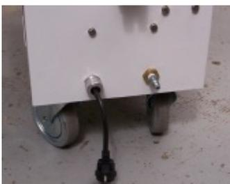
The electrical connection is located on the front (handle side) of the machine. The electricity is used to power the heater inside the cabinet. The electric heater requires less than 10 amps of 110v or 240v AC voltage.
