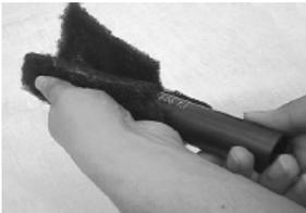
3. If the piston is scratched or marred, polish its surface with an abrasive cloth until no burr remains to damage the metering sleeve.
