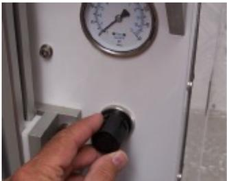
The pressure regulator at the front of the machine is adjusted by rotating to the right (clockwise) to increase the dispense pressure. Increasing the dispense pressure will increase the flow of material from the static mixer. Turning the regulator to the left (counter clockwise) decreases the dispense pressure. The knob locks into place when pushed in and must be pulled out to adjust the pressure.
