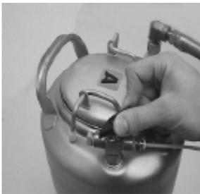
1. Rotate the selector valve pointer 180° from the air inlet tubing. This will close off incoming air, and vent the tank.
