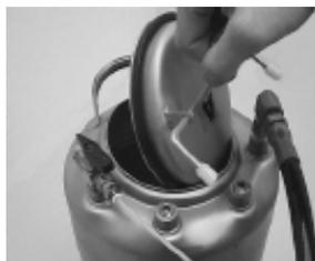
3. Twist and tilt the lid until it clears the opening. The lid seal should be attached to the rim. If not, check to see if it has dropped into the tank, or stuck to the underside of the tank lip.
